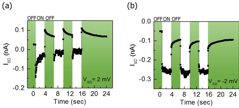
Figure S5. Time-resolved photocurrent of 1L-3L MoS<sub>2</sub> junction under small bias ( $V_{SD} = \pm 2$  mV).
