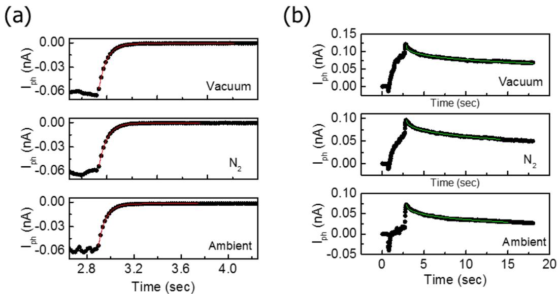
Figure S3. Time-resolved photocurrent measurement at (a) zero bias and (b)  $V_{SD} = 5\text{ mV}$  under different gaseous conditions. The red and green curves represent the fitting curves based on normal exponential decay and stretched exponential decay, respectively.
