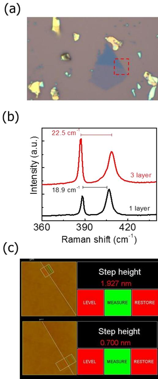
Figure S2. (a) Optical microscope image and (b) Raman spectra and (c) AFM image of 1L-3L MoS<sub>2</sub> junction (Sample A).
