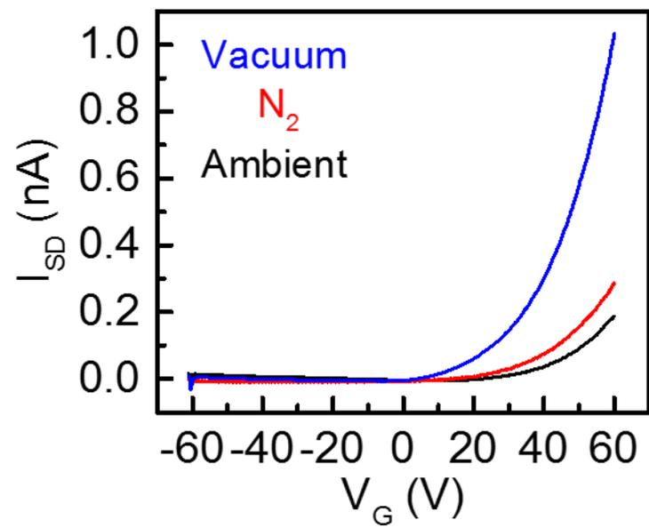
Figure S1. The transfer curves of 1L-3L MoS<sub>2</sub> junction device under vacuum, N<sub>2</sub>, and ambient conditions.
