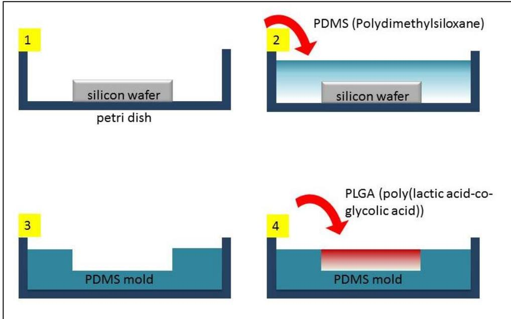
**Supplementary Figure 2:** Preparation of PDMS molds and poly(lactic acid-co-glycolic acid) (PLGA) (85:15) micropatterned films from SU-8 micropatterned array chiplets.
