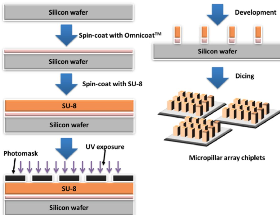
**Supplementary Figure 1:** Production of SU-8 micropillar array chip.
