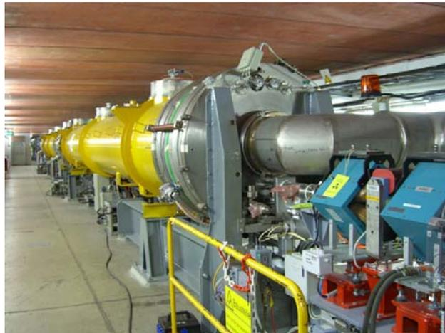
Figure S3: Superconducting accelerator of FLASH. Yellow barrels are superconducting modules with accelerating gradient up to 25 MV/m.
