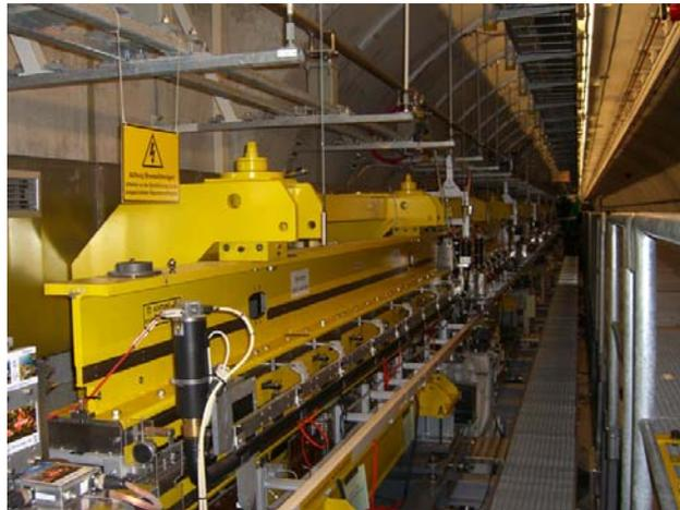
Figure S4: Undulator of FLASH is a permanent magnet device (period 2.73 cm, gap 12 mm, peak field 0.48 T). The undulator system is subdivided into six segments, each 4.5 m long. The vacuum chamber has 9 mm inner diameter.
