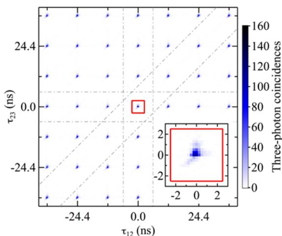
**Supplementary Fig. 2:** Three-photon coincidence map as function of the relative delays between detectors 1-2 (bottom axis) and 2-3 (vertical axis). The two-dimensional time bin for the coincidences detection is  $256 \times 256$  ps<sup>2</sup>.
