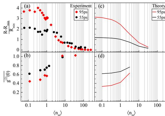
**Supplementary Fig. 1: Dependence on the pulse temporal length (Device 2).** (a) Measured reflectivity contrast as function of  $\langle n_{in} \rangle$  for 52 ps (black circles) and 94 ps (red diamonds) excitation pulses. (b) Measured second-order correlation measurements at zero delay for 52 ps (black circles) and 94 ps (red diamonds) excitation pulses. (c),(d) Corresponding calculated curves.
