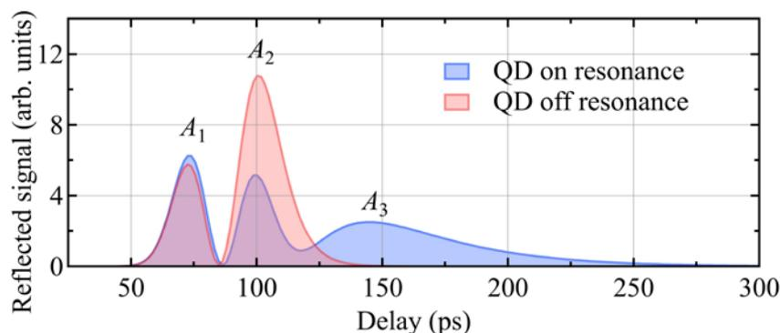
**Supplementary Fig. 4:** Simulation on the time evolution of the intensity reflected by device when the QD is on (blue curve) and off resonance (red curve).
