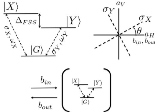
**Supplementary Fig. 3:** Supplementary figure 2: schematic of the model and notations. a: three level atomic system. b: relative orientations of the QD exciton axes and the cavity axes. c: input, output and cavity field operators.
