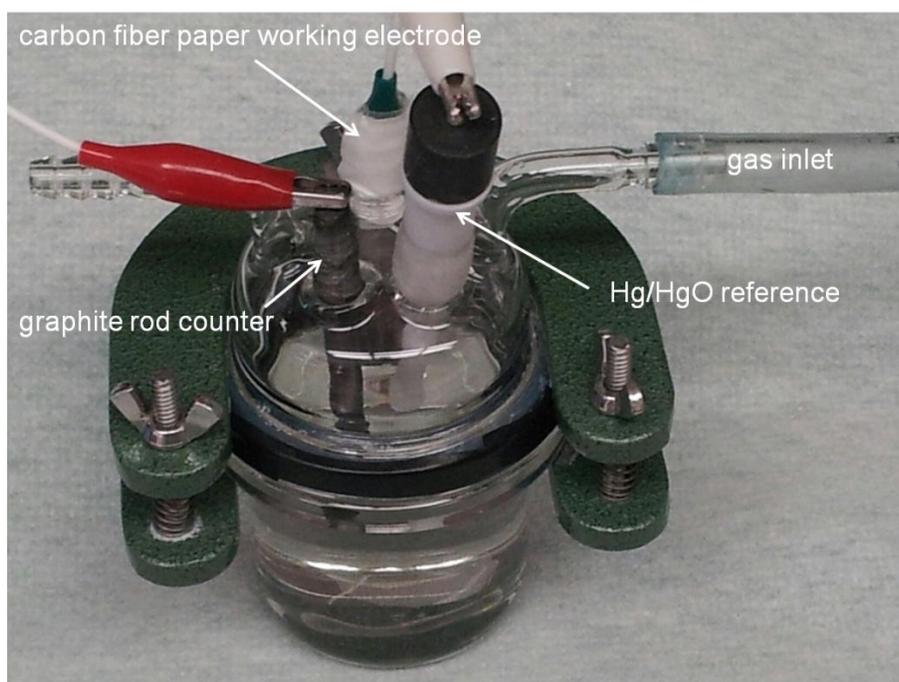
**Supplementary Figure S1.** Photo of our home-built electrochemical cell for the ORR and OER measurements. The three electrode system consists of an Hg/HgO reference electrode (filled with 6 M KOH), a graphite rod counter electrode and electrocatalyst loaded carbon fiber paper as the working electrode. The cell has a gas inlet that allows continuous O<sub>2</sub> purge when needed for ORR.
