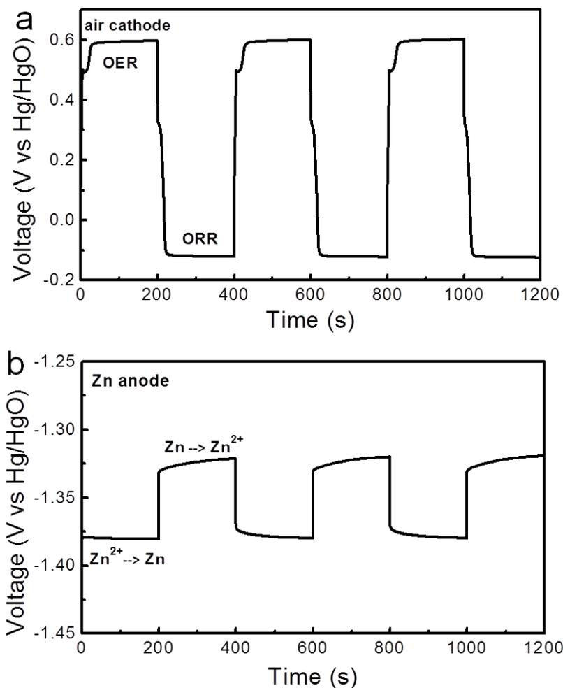
**Supplementary Figure S4.** Alternating oxidation and reduction of (a) the air cathode and (b) the Zn anode at a current density of 20 mA/cm<sup>2</sup>. Based on above data, the voltage polarization observed in Figure 5b of the main text was mainly contributed by the air cathode side (sum of ORR and OER overpotentials). Polarization on the Zn anode was negligible.
