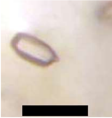
Supplementary Fig. 3. Fluid inclusion. Typical appearance of an all-liquid aqueous inclusion. Scale bar is 10 \mu\text{m} .
