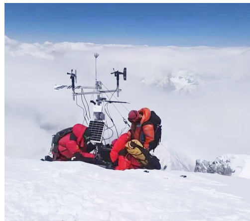
▲ UCAS Yanqi Lake Campus; STEP team members setting up the world's highest automatic weather station on the top of Mount Qomolangma.
