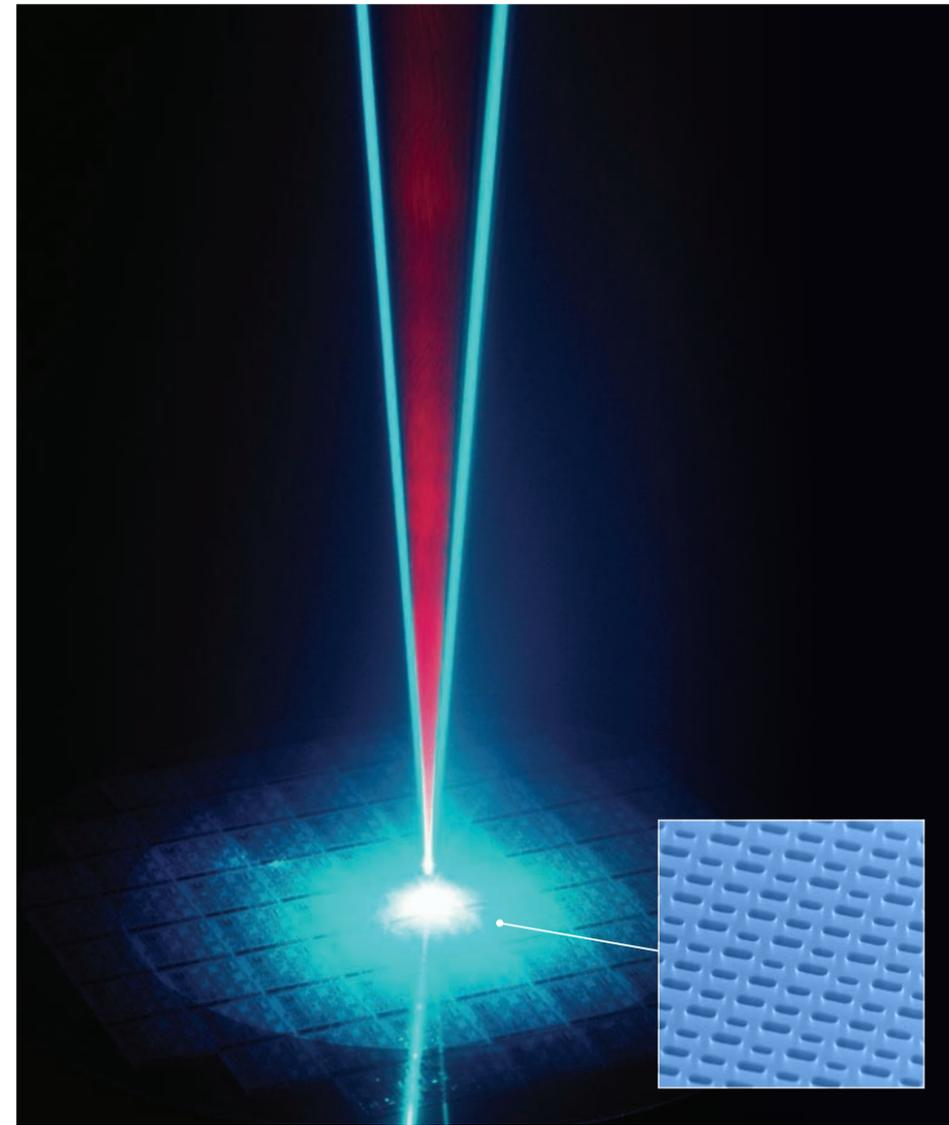
▲ Photonic-crystal surface-emitting lasers enable built-in beam-steering and beam-shaping functionality. The inset shows a scanning electron microscope image of a photonic crystal specially-designed for this purpose.
