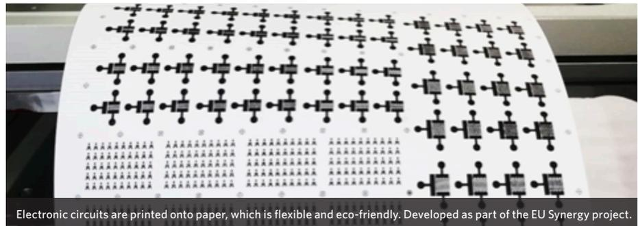
Electronic circuits are printed onto paper, which is flexible and eco-friendly. Developed as part of the EU Synergy project.
