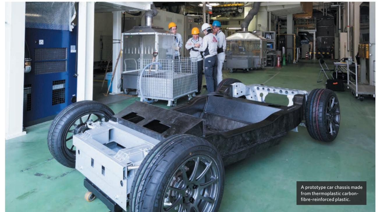
A prototype car chassis made from thermoplastic carbon-fibre-reinforced plastic.
