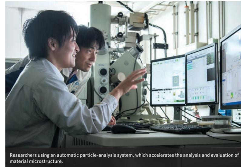
Researchers using an automatic particle-analysis system, which accelerates the analysis and evaluation of material microstructure.
