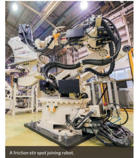
A friction stir spot joining robot.
