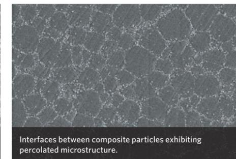
Interfaces between composite particles exhibiting percolated microstructure.
