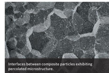
Interfaces between composite particles exhibiting percolated microstructure.
