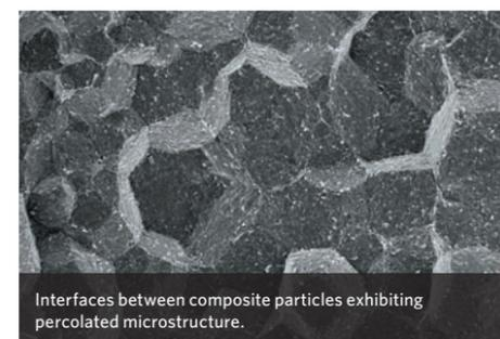
Interfaces between composite particles exhibiting percolated microstructure.
