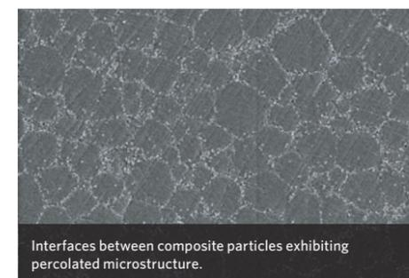
Interfaces between composite particles exhibiting percolated microstructure.
