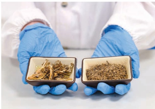
Post-fermentation prawn shells and powder with enriched chitin/chitosan.
