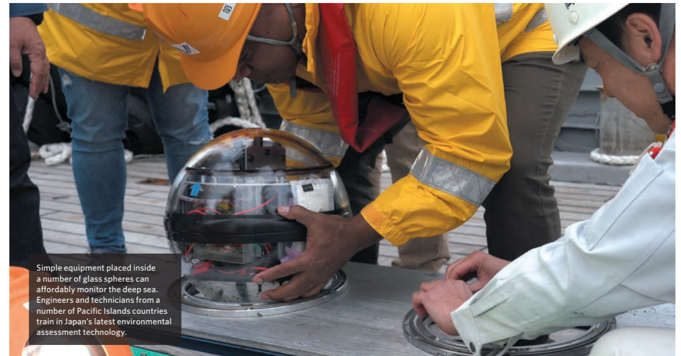
An Edokko Mark I type 365 sinks to the deep-sea bottom. It can be raised to the surface via an acoustic signal from a research vessel.
