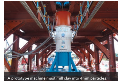
A prototype machine must mill clay into 4mm particles.
