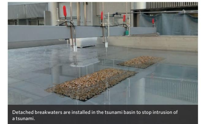
Detached breakwaters are installed in the tsunami basin to stop intrusion of a tsunami.
