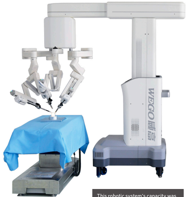
This robotic system's capacity was demonstrated via a remote operation to stitch up an eggshell membrane.
