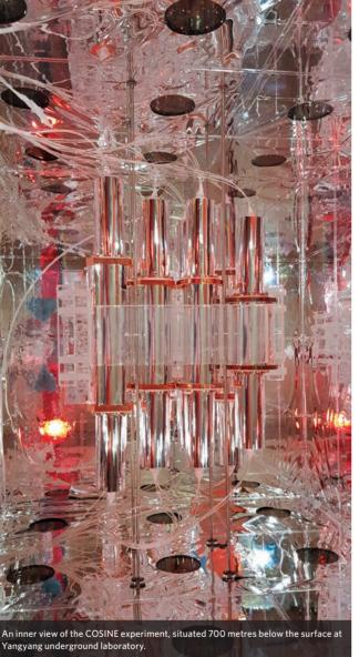
scintillating crystal medium. As other forms of ionizing radiation such as cosmic rays also cause these flashes, scientists house these crystals in lead boxes deep underground to shield the detector from anything but WIMPs.
