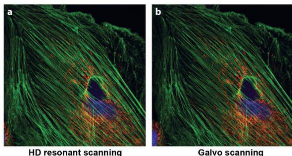
**Figure 2** | Comparison of image quality. **a,b**, Examples of the image quality achievable with the A1R HD25 resonant scanner (**a**) and a galvo scanner (**b**). Image quality is maintained with the resonant scanner. Both panels show the same area of a fluorescently stained endothelial cell from bovine pulmonary artery.
