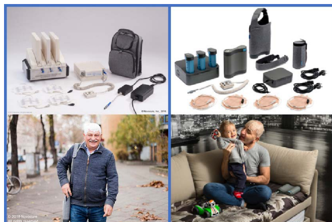
Figure 3: First and second generation Optune devices. The first and second generation Optune devices are comprised of two primary components: the electric field generator, preset to 200 kHz for GBM, and insulated transducer arrays incorporated in four bandages. The device treatment kit includes a plug-in power supply, portable battery, battery rack, battery charger, connecting cables and carrying case. Design changes in the second generation device using improved electronic components, circuit boards and digital signaling technology, resulted in reduced weight and increased operational efficiency for people with glioblastoma multiforme, improving the patient experience with TTFields treatment. (Top left, 1 st generation Optune; Top Right, 2 nd generation Optune; Bottom panels, patients wearing 2 nd generation Optune with white and tan arrays).
