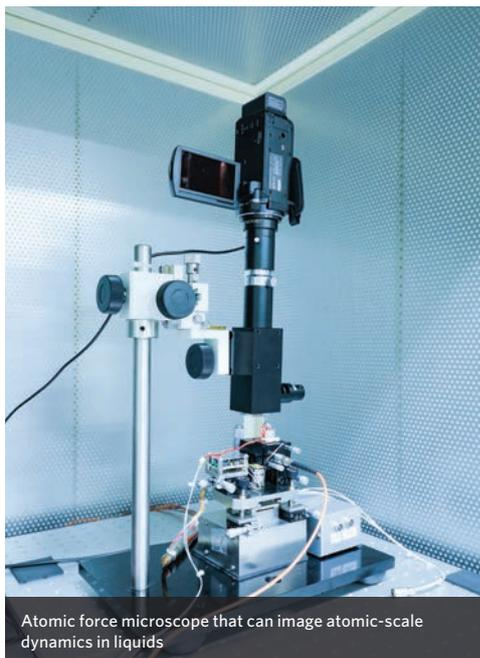
Atomic force microscope that can image atomic-scale dynamics in liquids
