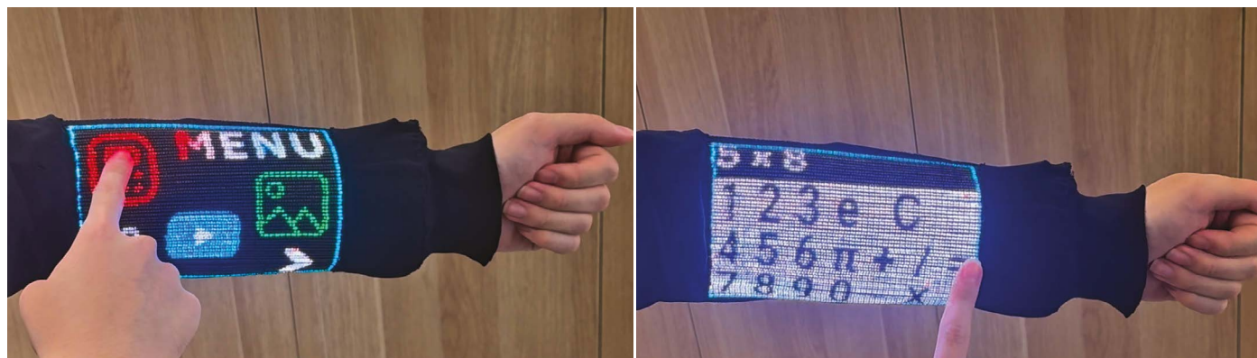
Figure 1 | A textile that acts as a graphical user interface. Fu et al. 1 report a graphical user interface made from light-emitting, pressure-sensitive fibres. The device has the flexibility and breathability of conventional fabric and was integrated into the sleeve of a garment. It responds to touch and executes various functions, including acting as a calculator.
