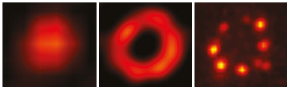
Nuclear pores seen using a form of ultrastructure expansion microscopy (right) compared with no expansion (left) and a type of super-resolution microscopy (middle).
