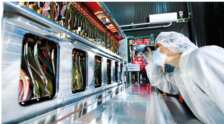
The LHCb’s ‘vertex locator’, placed close to the LHC’s beamline to see short-lived particles.
