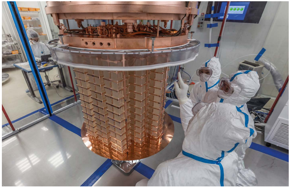
Figure 2 | The CUORE experiment involves a cubic-metre array of tellurium oxide crystals.
