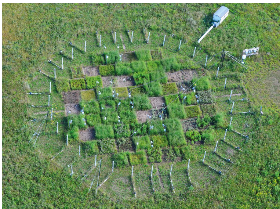
Figure 1 | A free-air CO 2 enrichment (FACE) experiment at the Cedar Creek Ecosystem Science Reserve in Minnesota. CO 2 -enriched air is emitted from the vertical vent pipes to simulate artificial CO 2 levels for plants growing under realistic field conditions.
