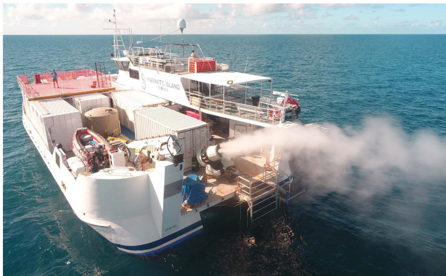
During a field trial, a turbine generates plumes of seawater droplets that rise into the sky.
