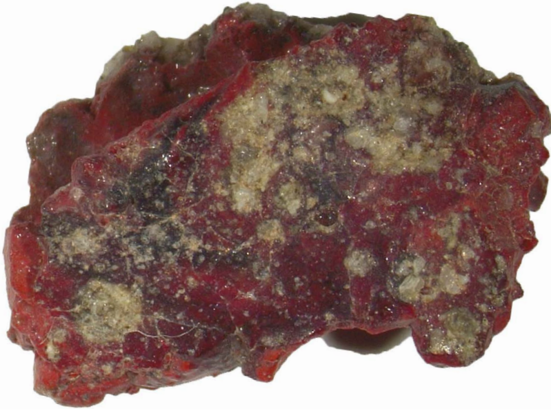
This sample of red trinitite was found to contain a previously unknown type of quasicrystal.
