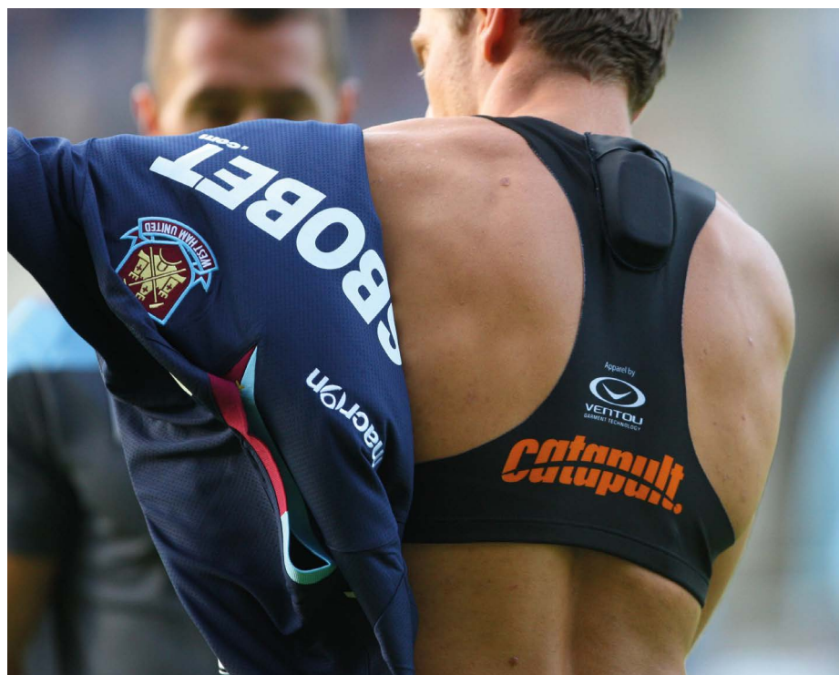
A football player wears a vest holding a GPS sensor. The data captured feed into an algorithm.
