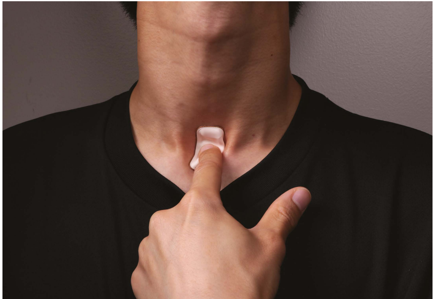
A soft, flexible device worn on the throat continuously measures and interprets coughing and breathing rates in people with COVID-19.
