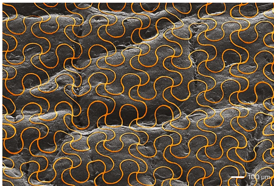
Microscope image of a flexible circuit printed onto skin, which works even when stretched.
