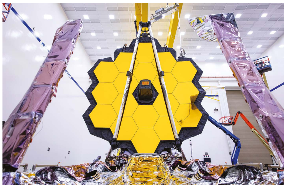
The James Webb telescope. Its mirror and sunshield will be folded up during launch.
