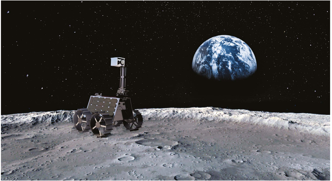
An artist's impression of Rashid, the UAE's lunar rover, which will include high-resolution cameras, a thermal imager and a Langmuir probe.
