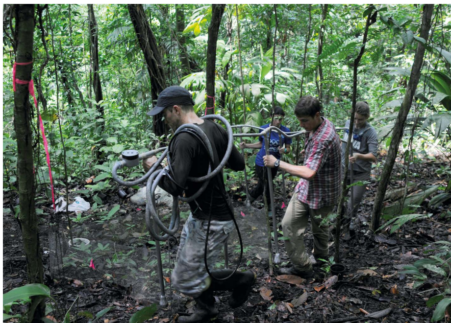
Figure 1 | Preparing to use a heating device in an experiment. Nottingham et al. 3 buried heating equipment in plots in a tropical forest in Panama and monitored the affect of warming on carbon dioxide release from the soil.
