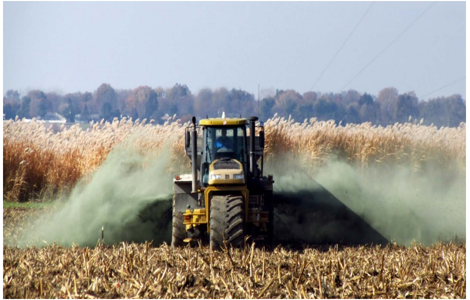
Figure 1 | Application of silicate material to cropland. Beerling et al. 1 demonstrate that enhanced rock weathering, achieved by adding crushed basalt or other silicate material to soil, is an effective strategy for removing carbon dioxide from the atmosphere.
