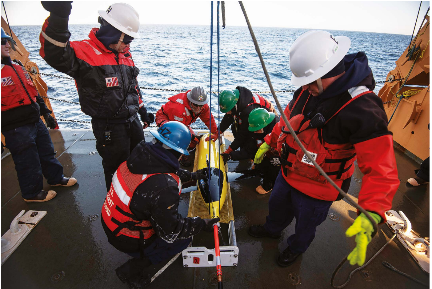
A sea glider being hoisted onto a ship in the Arctic Ocean after taking various measurements, including of conductivity, temperature and depth.
