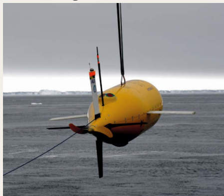
Autosub can record data beneath ice shelves.
