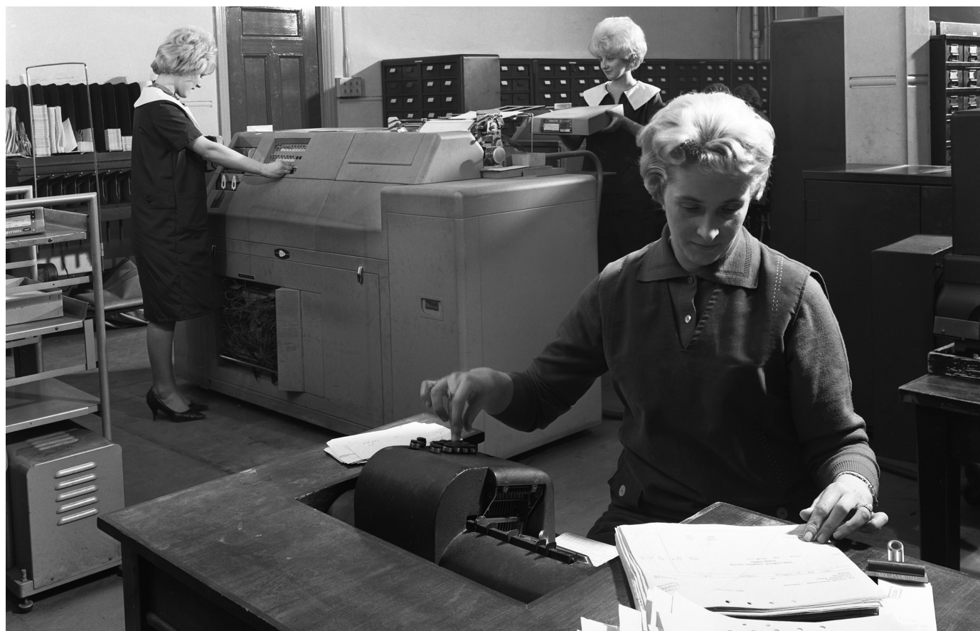
A Hollerith data machine at a steel works in Sheffield, UK, in 1963. The electromechanical device helped workers to tabulate statistics stored on punch cards.
