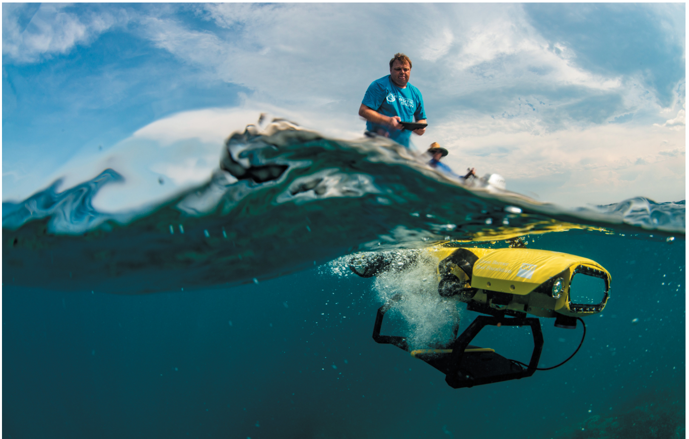
A tethered robot — LarvalBot — disperses coral larvae on 3 hectares of the Great Barrier Reef.
