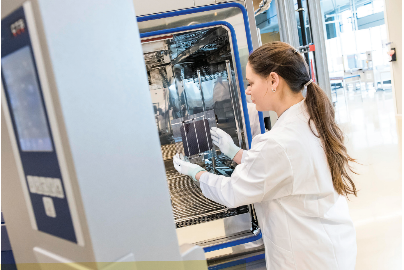
A researcher at Oxford PV's pilot production facility in Brandenburg an der Havel, Germany, tests a commercial-size solar cell made by layering perovskite on silicon.
