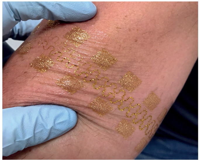
A flexible circuit designed to capture electrical signals from muscle activity.
