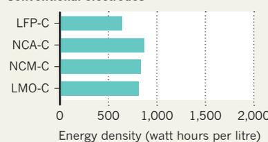
C, carbon (graphite); LFP, lithium iron phosphate; NCA, lithium nickel cobalt aluminium oxide; NCM, lithium nickel cobalt manganese oxide; LMO, lithium manganese oxide.
