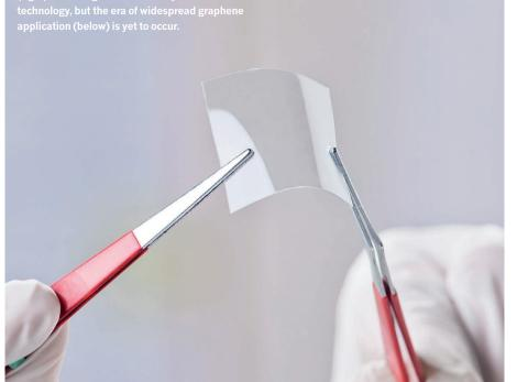
made headlines with a new production method that synthesizes graphene on top of a reusable layer of germanium, which guides the crystal growth to keep the structure uniform. The resulting graphene forms a single crystal big enough to be useful in electronics. The study was published in *Science*.
