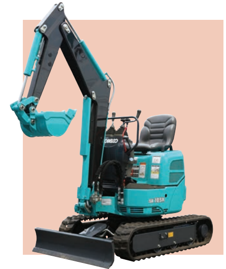
Excavator equipped with a lightweight Taguchi attachment.
