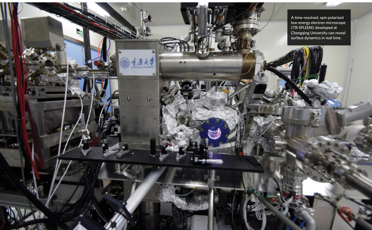
A time-resolved, spin polarized low-energy electron microscope (TR-SPLEEM) developed at Chongqing University can reveal surface dynamics in real time.
