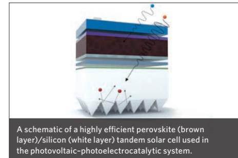
A schematic of a highly efficient perovskite (brown layer)/silicon (white layer) tandem solar cell used in the photovoltaic-photoelectrocatalytic system.
