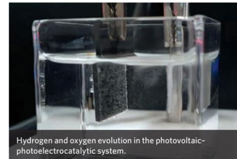
Hydrogen and oxygen evolution in the photovoltaic-photoelectrocatalytic system.
