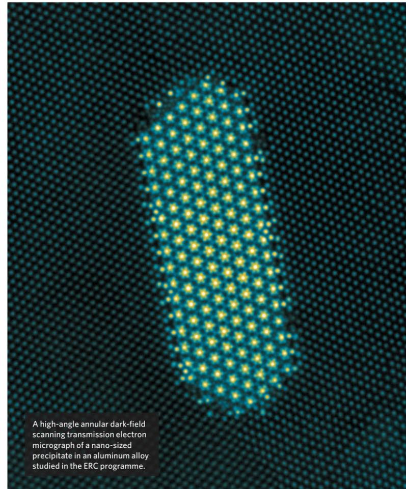
A high-angle annular dark-field scanning transmission electron micrograph of a nano-sized precipitate in an aluminum alloy studied in the ERC programme.
