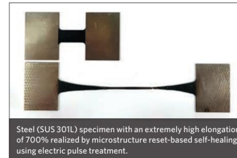
Steel (SUS 301L) specimen with an extremely high elongation of 700% realized by microstructure reset-based self-healing using electric pulse treatment.
