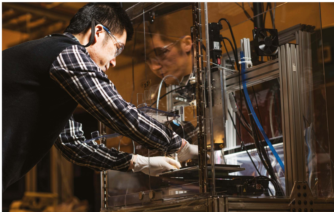
Chemist Ying Zhu places a nanoPOTS chip containing protein samples into an automated analysis system.
