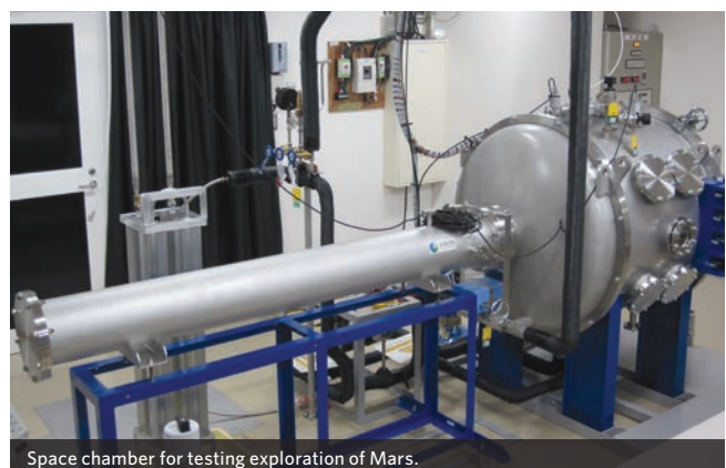
Space chamber for testing exploration of Mars.
